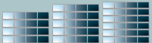
4 sections Doors up to 2280mm high. 5 sections Doors up to 2835mm high. 6 sections Doors up to 3000mm high.
